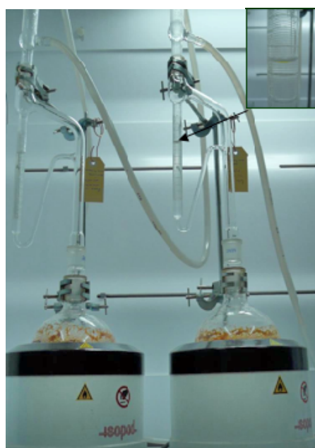
Figure 1. Dean-Stalk apparatus used for hydro-distillation of the sandalwood oil from milled heartwood.
